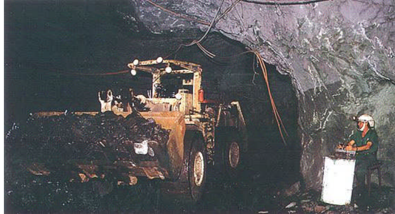
Fig 13: A Remote-Controlled Load-Haul Dump Machine Moving Ore from Stopes to an Orepass, Olympic Dam Copper-Uranium Mine, Woomera, SA (photo courtesy of www.mining-technology.com ).
