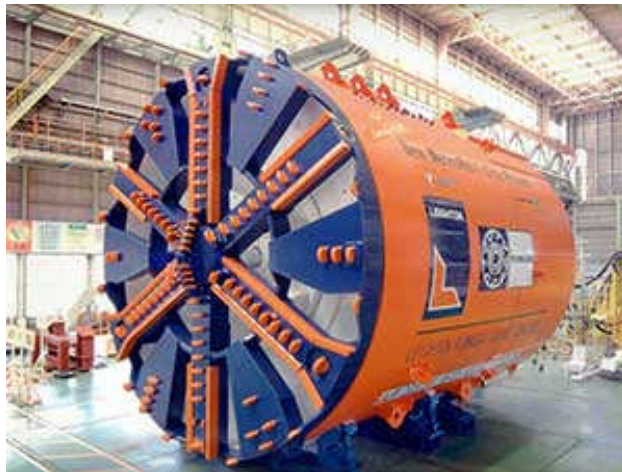
Fig 20: NewMetroRail City Project, Perth WA - 7.0 m diameter TBM Shield (Sandgroper) (photo courtesy of Australian Tunnelling Society).
