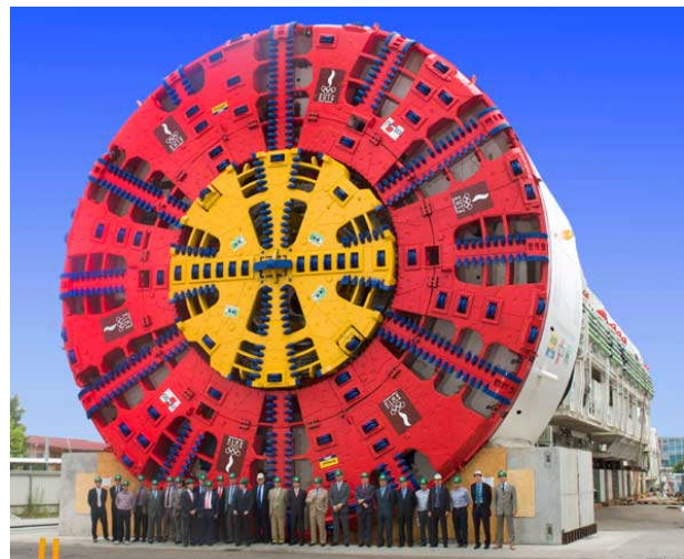
Fig 27: The largest TBM currently in operation is a Herrenknecht 15.2 m diameter, 4,364 t S-300 EPB machine being utilised on a 3.65 km long motorway tunnel in Madrid (photo courtesy of Herrenknecht AG).
