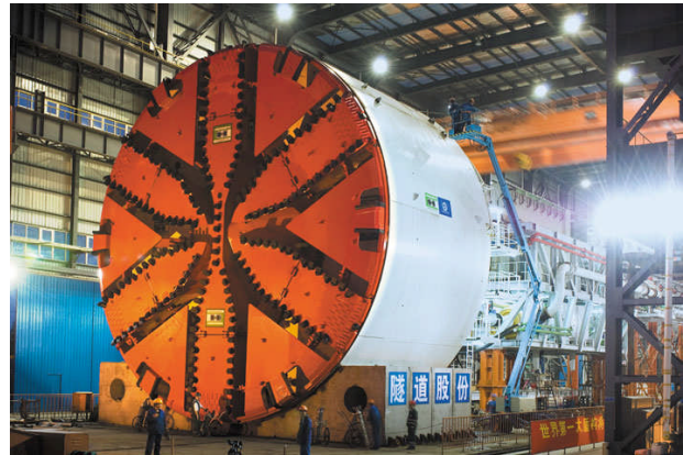
Fig 28: Herrenknecht are currently commissioning a 15.43 m diameter S-317 mixshield in Shanghai where it will be used to construct one of two 7.2 km long three lane road tunnels (photo courtesy of Herrenknecht AG).
