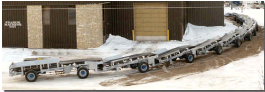
Fig 40: Prairie Machine Parts Flexiveyor Continuous Haulage system (photo courtesy of Prairie Machine Parts).
