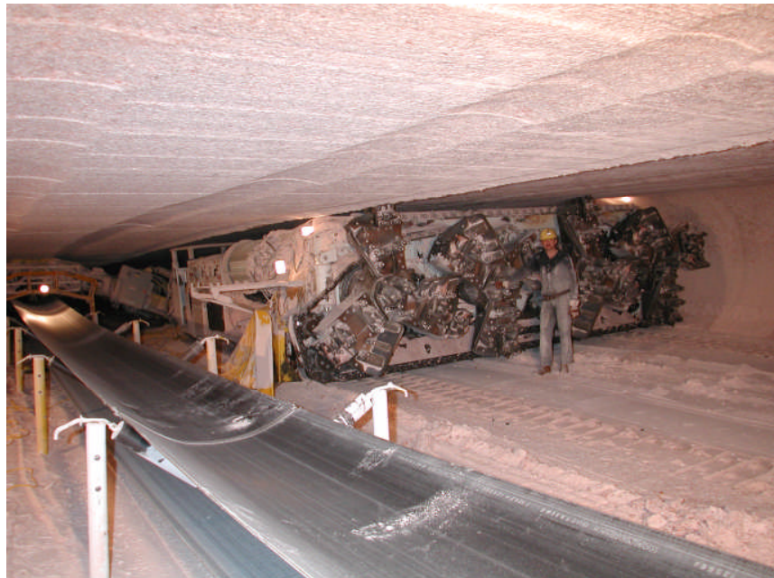
Fig 39: Prairie Machine Parts Xcel-44 Four Rotor 400 hp Borer Miner Underground at Saskatoon, Canada (photo courtesy of Prairie Machine Parts).
