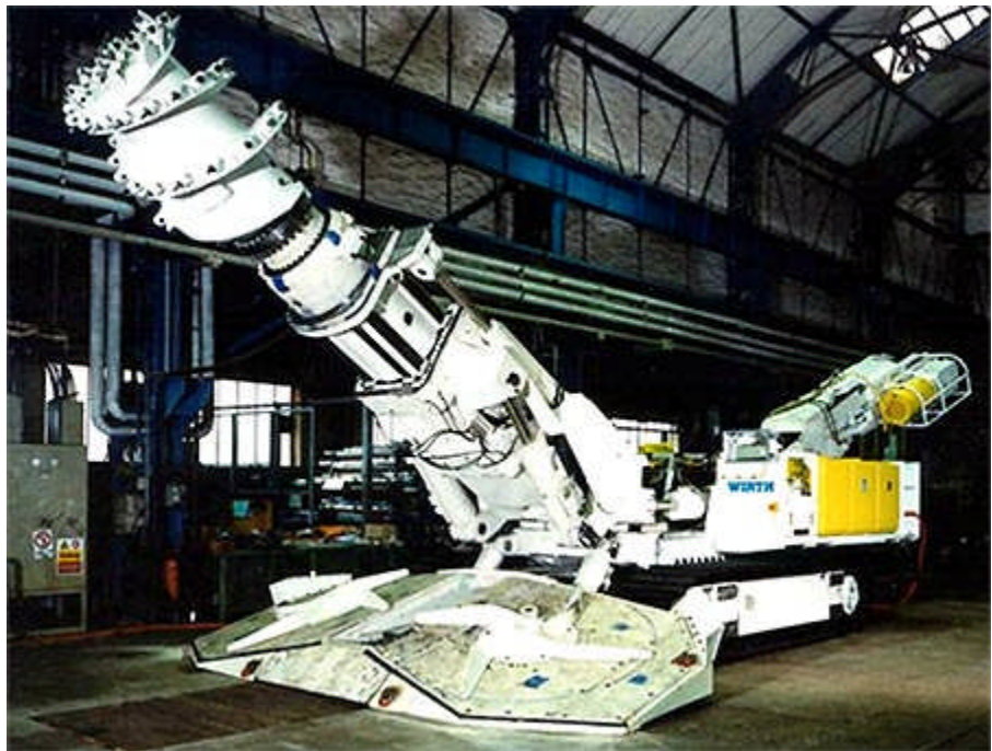
Fig 42: Wirth T4.31 Continuous Mining Machine, Designed for the Continuous Extraction of Minerals such as Salt, Potash, or Gypsum (photo courtesy of www.mining-technology.com )
