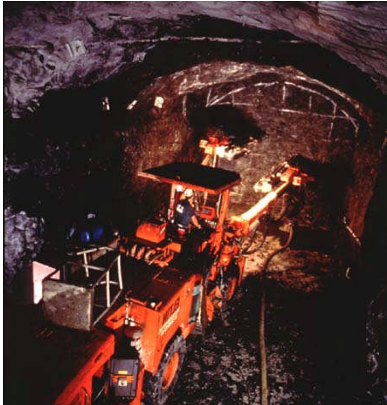
Fig 6: Tamrock Minimatic Two-Boom Jumbo in Development of Access Decline at Kanowna Belle Gold Mine, Kalgoorlie, WA (photo courtesy of www.mining-technology.com ).
